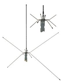
25 -1200 MHz - Ideal for all band scanners: low band, high band and UHF frequencies ● 4 Sets of specific frequency stainless steel radials (21" – 2 Meter, 13.75" – 1.25 Meter, 5.25" – 70 cm, 3" – 33cm) ● Copper wound fiberglass center element for low frequencies ● Mounts on 1-1/4" to 2" mast pipe ● Antenna connection: SO-239 ● Available with 50' or 75' of low loss coax cable & BNC connectors
