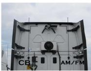
Mounts on the back of the truck cab ● Kit includes: 5 FT AM/FM antenna, Back of cab mount, 19 FT RG62 cable, Antenna guide & mounting hardware
